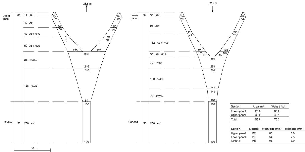
**Figure 2.** Crustacean trawl design utilized during experimental fishing.
