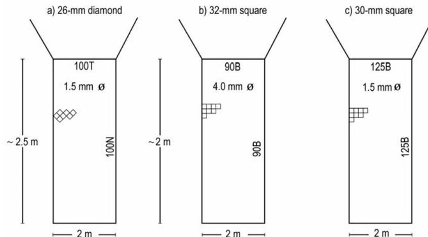
**Figure 2.** Diagrammatic representation of a) the control 26 mm diamond-shaped mesh polyamide-PA codend, b) the 32 mm square-mesh (22.5 mm outside bar) polyethylene-PE codend, and c) the 30 mm square-mesh (16 mm outside bar) polyamide-PA codend used in the experiment (T: transversals, B: bars, N: normals).
