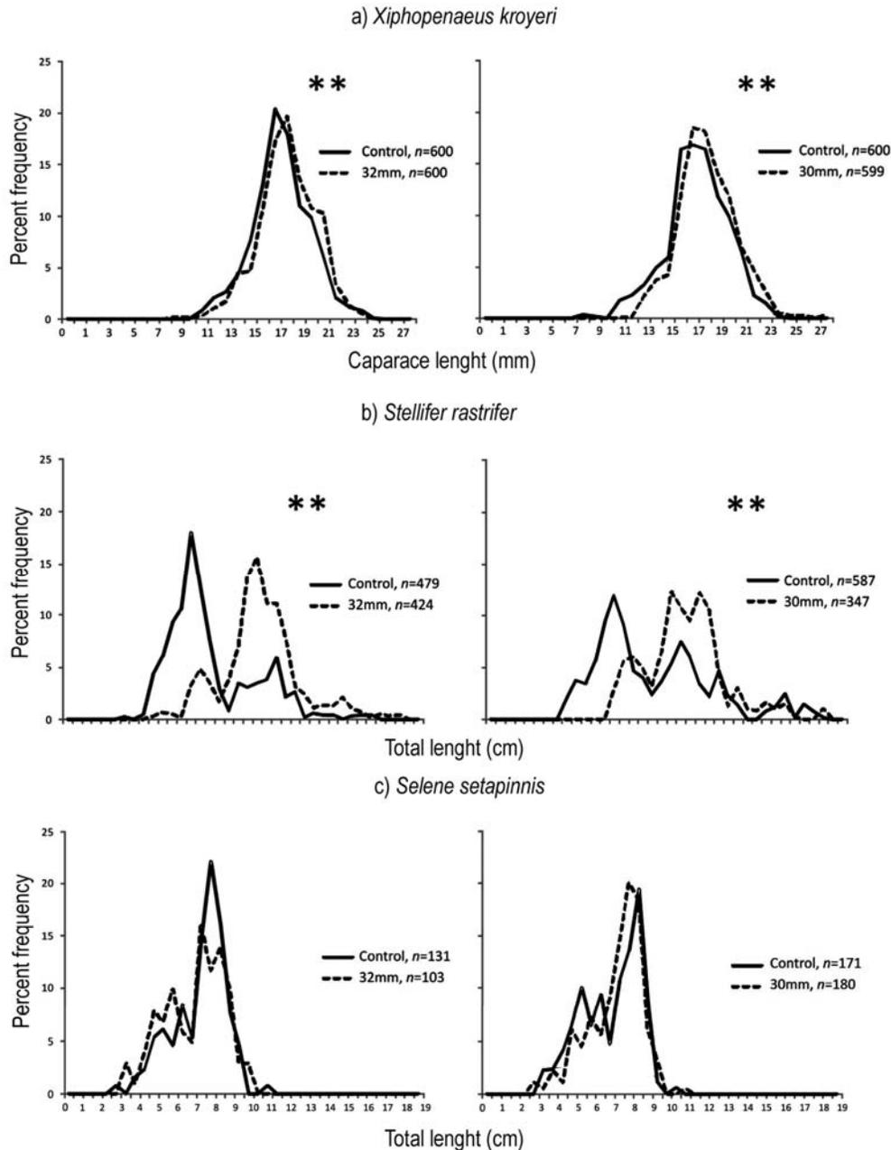
**Figure 4.** Size-frequency distributions of a) *Xiphopenaeus kroyeri*, b) *Stellifer rastrifer*, and c) *Selene setapinnis* captured with the control and square-mesh codends (32 and 30 mm) during the experiment. \*\* Significant differences at  $P < 0.01$ .
