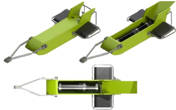
**Figure 10.** U-Tow II in open and closed views.
