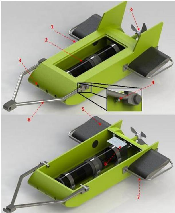
**Figure 8.** U-tow. 1) Body of the vehicle in fiberglass, 2) multiparameter probe, 3) hole for entry of continuous flow of water, 4) safety pin, 5) hydrofoil, 6) gearbox, 7) hydrofoil guard, 8) tow hitch, 9) variable speed propeller.
