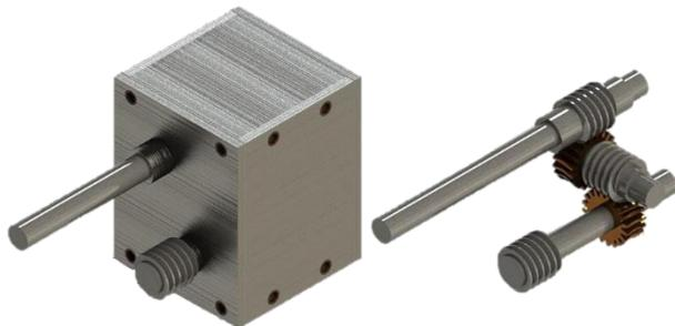
**Figure 4.** Simplified 3D Model of the gear (100:1) between the propeller and the undulator.
