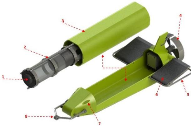
**Figure 14.** U-Tow IV. 1) Multiparameter probe, 2) mounting track, 3) transport box, 4) propellor guard, 5) hydrofoil guard, 6) hydrofoil, 7) inputs to the continuous flow of water, 8) tow hitch.
