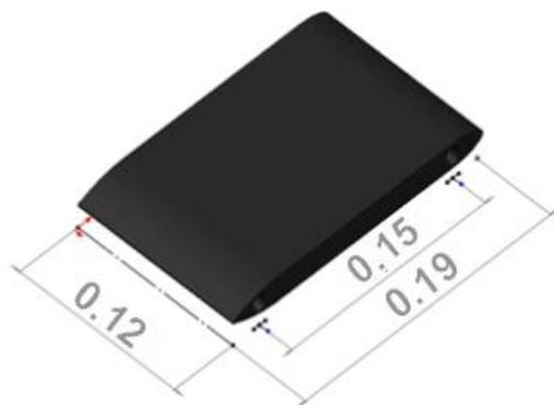
**Figure 5.** Isometric hydrofoil NACA 0012.
