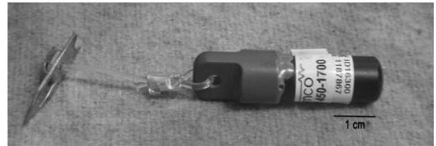
**Figure 2.** External anchoring system for the Vemco V9-2H ultrasonic transmitter. The stainless-steel dart tag FH-69 (Floy-Tag) modified and reduced and attachment to the transmitter are shown.
